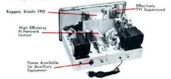
**TUNING** — The "Valiant's" basic tuning controls are located on the VFO dial escutcheon. QSY within the phone or CW portion of a band is usually possible by merely changing the VFO frequency setting. For larger frequency excursions, simply touch up the exciter tuning, adjust loading, and dip the final.
